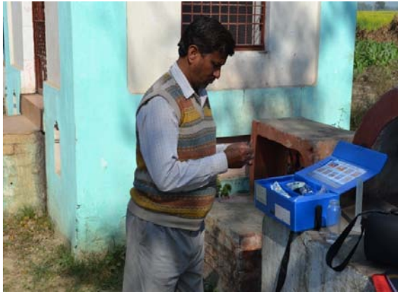
Arsenic testing of water sample by FTK
