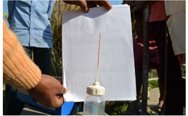
Red colour shows the presence of Arsenic in water sample.
